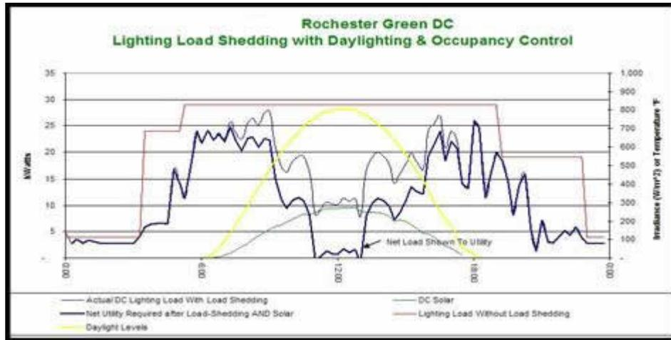
Figure 6 - Power Consumption by DC Lighting System
